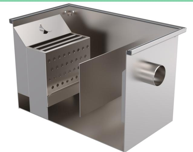
With the food particles settling on the base, and the grease trapped on the surface behind the last baffle wall, grease is prevented from entering the waste discharge
