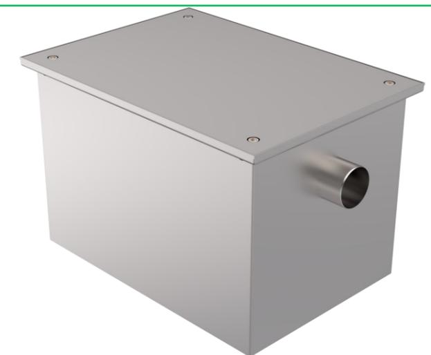
Internally, the large first baffle slows the water down. This will help the discharge to cool enough for the grease to lose momentum and rise to the surface of the water. The perforated baffles also helps Food Particles to separate from the Water and the FOGs, and to settle on the bottom
