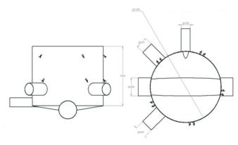
Liner sizes are customised to suit each project - the following are examples of previous sizes manufactured and can be completely adapted in terms of height/width/dept/ and inlets size and quantity.
