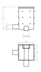
Liner sizes are customised to suit each project - the following are examples of previous sizes manufactured and can be completely adapted in terms of height/width/dept/ and inlets size and quantity.
