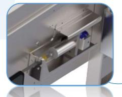
All machines are supplied with a **spring pack tension system for optimal belt alignment on the rollers.** There is no steering but there are guides within the machine to track the belt. Filtrate drains to the bottom and out through the filtrate outlet.
