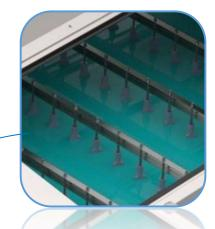
Sludge is spread across the full belt width. Sludge ploughs furrow the sludge as it is processed allowing free area on the belt for maximum filtrate drainage.
