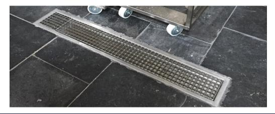
Specify: Kent Plain Mesh Grating KMG $\underline{150}$ ;  $\underline{150mm}$  wide grating;  $\underline{990mm}$  long; Grade  $\underline{304}$  Stainless Steel; Load Class  $\underline{B}$
