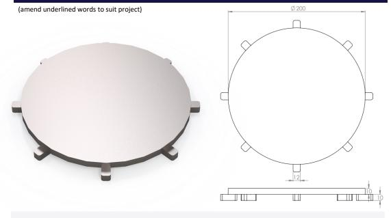
Industrial Annular Channel Grating is typically supplied with the KV250 Family of Round Top Drain Gullies
