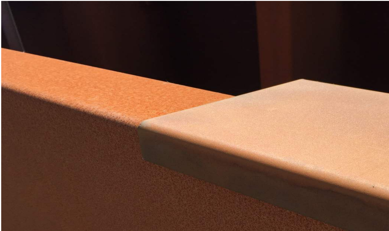
Pre Weathered Corten (left) VS Imitation Corten
