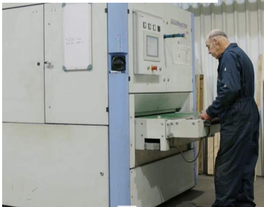
Flat Bed Polishing with 320 Grit Belts
